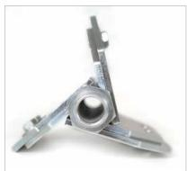
DN 200-450 centralizer with 2 sets of adjustable position skids. Steel wheels are set on bigger skids. Suitable for 1" nozzles (Tremol, Rondò, Warthog, Friuli, Maniago).
